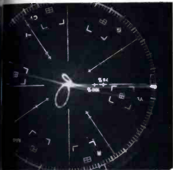
Fig. 1 Expanded center of color bar showing "Bow Tie" leading edge of grey bar (No. 1) and modified "Bow Tie" sync (No. 2). Note absence of jitter both with respect to other and also over the two-field period of the exposure.
