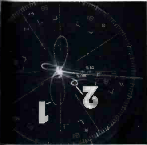
Fig. 1 Expanded center of color bar showing "Bow Tie" leading edge of grey bar (No. 1) and modified "Bow Tie" sync (No. 2). Note absence of jitter both with respect to other and also over the two-field period of the exposure.
